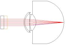
Next, I set the Zemax model wavelengths to 0.4, 0.45, 0.5, 0.55, 0.6, 0.65, 0.7  $\mu$ m to cover the visible region. I created a merit function to target the y height of a paraxial ray on the retina to be zero for each of these wavelengths. I set each surface of the plates to be variable. The plates are assumed in contact, so the middle surface will have the same shape ultimately for each lens. Optimizing this arrangement gives
