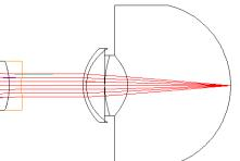
where the radii of the doublet are 17.290, -11.627 and 24.752 mm respectively. The longitudinal chromatic aberration of eye with and without the doublet is shown below.
