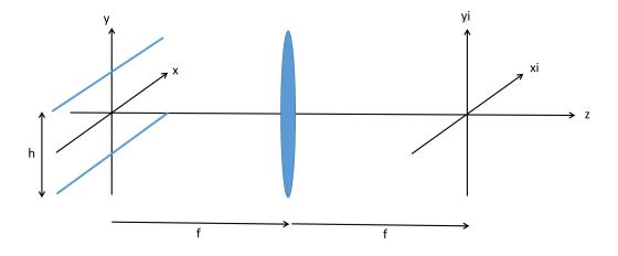
b) Calculate the irradiance pattern  $I_i(x_i, y_i, 2f)$  on the screen. You can ignore the effects of the pupil of the lens, and be sure your answer is in terms of coordinates  $(x_i, y_i)$ . *The field on the screen is given by*
