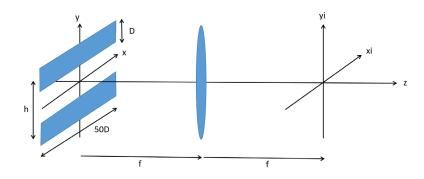
From the diagram, it should be evident that  $D/2 \le h/2$ , otherwise the openings start to overlap and give an impossible transmission value of 2 in the overlap regions. Thus
