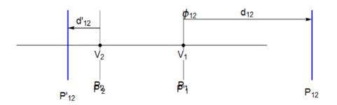
8. A system consists of two thin lenses separated by a distance of 8 mm. The focal length of the first lens is 3.75 mm and the focal length of the second lens is 10 mm. An object is located 4 mm to the left of the first lens. The object has a height of 0.5 mm.
