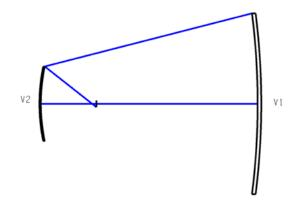
(b) Using Gaussian reduction, find the overall focal length of the telescope.
