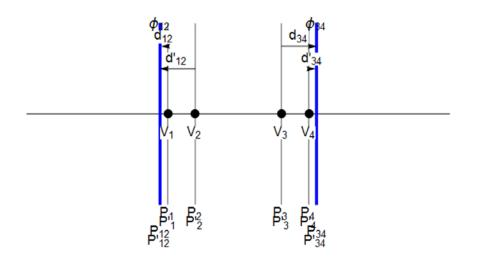
Next, we need to calculate the distance between these two reduced systems. The new distance  $t'_{12}$  is the separation between the rear principal plane of the first system  $P'_{12}$  and the front principal plane of the second system  $P_{34}$ . This distance is given by
