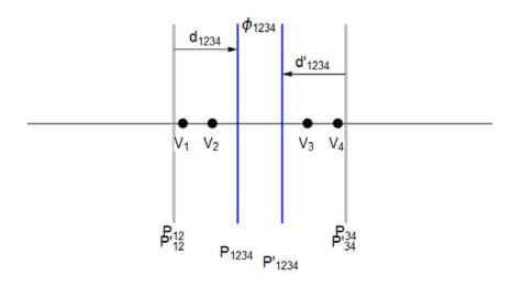
The effective focal length is  $f_E = \frac{1}{\phi_{1234}} = 40.29 \text{ mm}$ . The front and rear focal lengths are  $f'_R = 40.29 \text{ mm}$  and  $f_F = -40.29 \text{ mm}$ .
