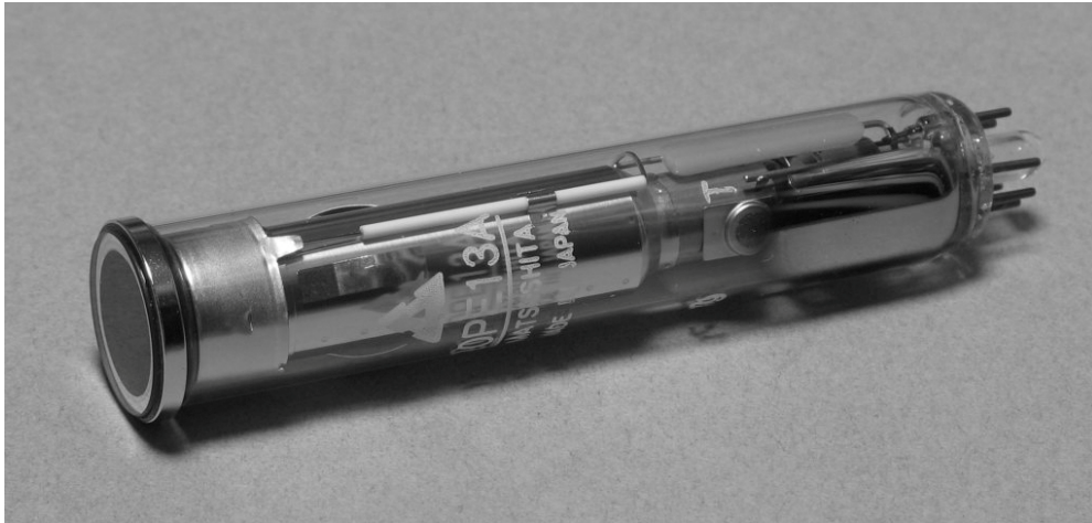
Figure 1-13 Vidicon tube. An image is projected onto the circular region at the left end of the tube leading to variations in capacitance on the surface. An electron beam within the tube scans across this surface and the resulting voltage variations encode the image.
