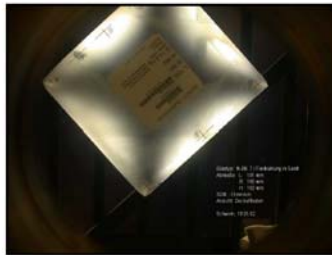
Figure 8: N-BK7 block with internal stress.
