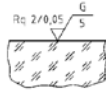
Figure 1 — Indication for ground surface with 2 \mu\text{m} > Rq > 0,05 \mu\text{m} and minimum sampling length of 5 mm
