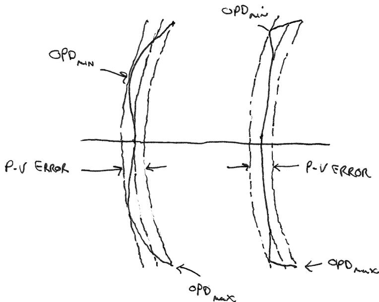
Both of these wavefronts have the same P-V error, but the one on the right is smoother except at the very edges. P-V tends to underestimate performance for systems with localized errors.
