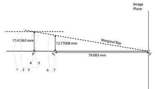
The height of the marginal ray at the first surface is 17.41365 mm and the height of the marginal ray at the last surface is 13.77008 mm. Based on similar triangles
