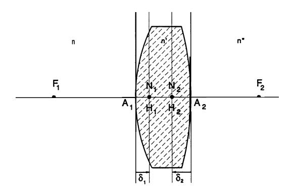
Figure 6.5. Cardinal points of a thick lens.
