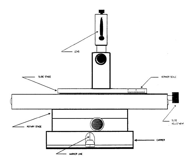
Figure 6.7. Nodal slide-mechanical layout.
