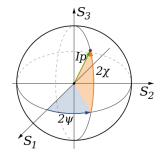
The equator contains all linear polarizations, while circular polarizations lie at the two poles. All other states are elliptical polarized. In this illustration one can imagine the action of a half-wave plate to be traversal in the azimuthal direction (moving along the equatorial direction at whichever latitude you start at) while the action of a quarter-wave plate is to alter the altitude
