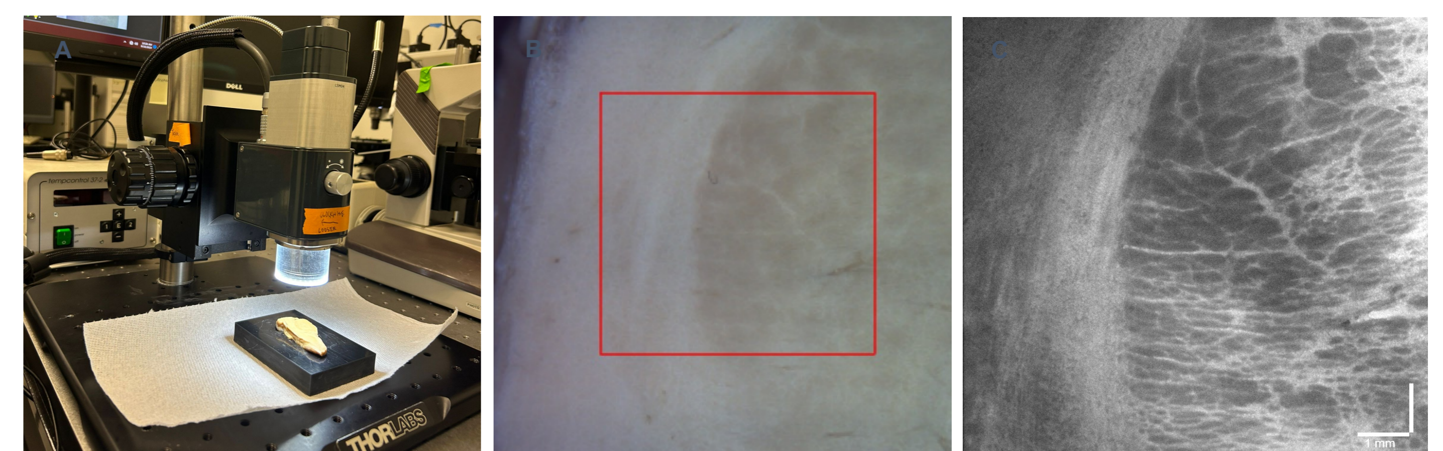
Figure 4. (A) PS-OCT set up. (B) Selected ROI. (C) Average intensity of the ROI obtained with PS-OCT.
