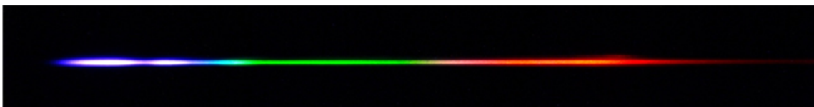
Figure 4. Super-continuum of laser light generated from short pulses sent through a nonlinear micro-structured fiber. A zoomed-in look at this spectrum would reveal a discrete frequency comb structure rather than a continuous distribution of frequencies.
