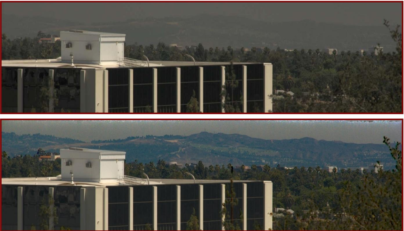
*Figure 11: Imaging through haze. Top: Image obtained with a linear polarizer optimally aligned for maximum contrast. Bottom: Image resulting from applying a dehazing algorithm to the Stokes image. Haze has a different polarization signature than the desired image, so its removal is far more effective when its polarization behavior is measured. (Images obtained by JPL.)*
