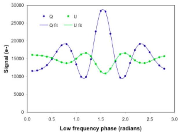
Figure 4: Detected signal at the beat frequency of the photoelastic modulators is a Bessel function.  $I$ ,  $Q$ , and  $U$  are extracted from a fit to Bessel function parameters.
