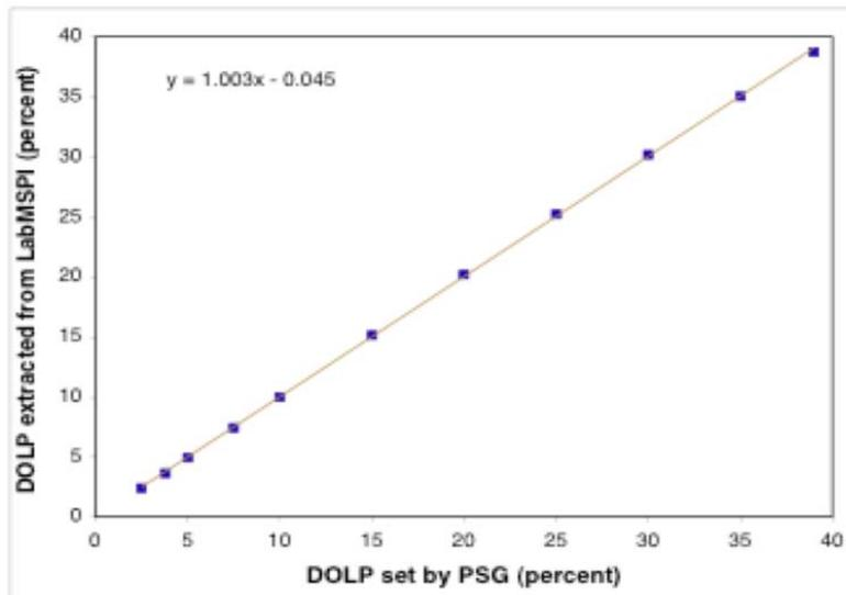
Figure 5: DoLP of Ground MSPI matches DoLP set by the PSG to an accuracy of 0.05%, too small to be visible on this graph.
