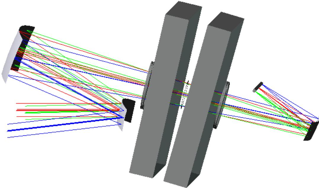
*Figure 2: MSPI schematic: Three curved mirrors form an off-axis astigmat. The large blocks are photoelastic modulators placed between achromatic quarter wave retarders. Filters and polarizers are integrated on the focal plane assembly.*
