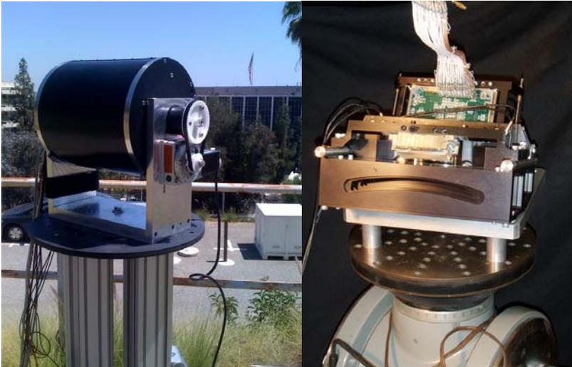
Figure 3: Ground MSPI mounted for outdoor observations (left) and with cover removed (right)
