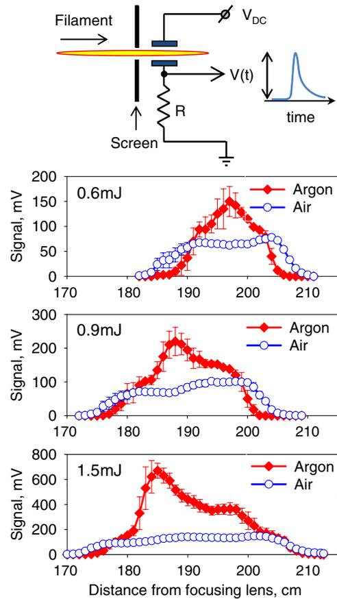
FIG. 1 (color online). Top panel: Schematic of the capacitive plasma probe. Bottom panels: Experimental data for plasma density generated through filamentation in air and argon under identical conditions, for three different values of pulse energy.
