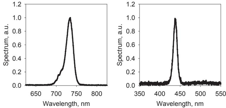
Fig. 2. Normalized spectra of the generated third and fifth harmonics on linear scale.
