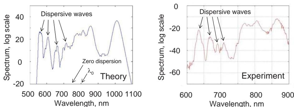
Fig. 2. Calculated (left) and measured (right) supercontinuum spectrum generated after propagation of an input Airy pulse with peak power of 1.6kW through 1 m of highly nonlinear fiber. The effective mode size of the fiber is  $2\mu\text{m}$  and zero dispersion wavelength is 750 nm. The center wavelength of the input pulse is 800 nm.
