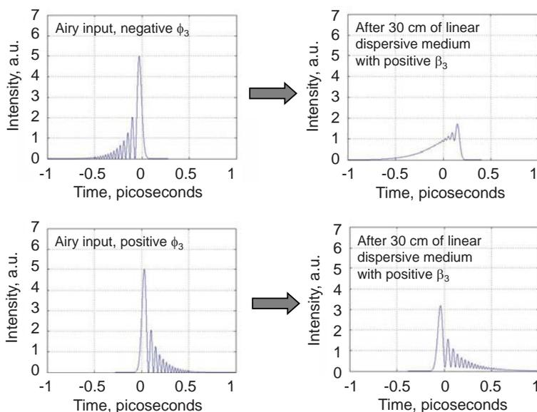
Fig. 1. Numerically simulated input Airy pulse and output pulse waveform after linear propagation through a dispersive medium representing the microstructured optical fiber used in the experiments. The range of distortion-free propagation of the pulse depends on the sign of the initial cubic spectral phase.
