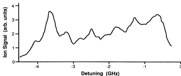
FIG. 3. Integrated ion signal vs trap-laser detuning for  $\Delta_{\text{molasses}} = -8.5$  MHz.
