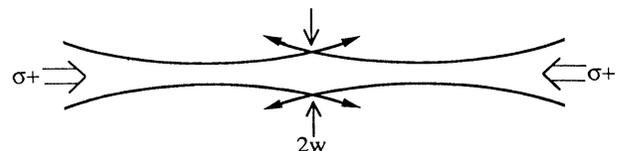
FIG. 1. Sketch of the trap geometry (not to scale). Foci of the two beams are separated by about the confocal parameter. Stable trapping is achieved at the midpoint between the foci where the waist ( $1/e^2$  radius of intensity) is  $w$ .
