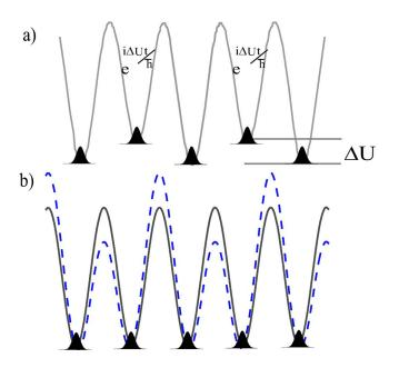
FIG. 5. (Color online) Lattice imperfections causing (a) modulation of the lattice depth,  $\Delta U$ , between neighboring sites and (b) state dependent modulation of the barrier height by a polarization lattice. In (b) the solid line is the cross section of the intensity lattice; the dashed line is the cross section of the state dependent lattice resulting from unbalanced beam intensities. Atoms in the ground state of each well are shown schematically.
