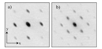
FIG. 7. Experimental images of atom diffraction from a  $3-\mu s$  pulse of (a) the in-plane lattice and (b) the out-of-plane lattice after 13 ms time of flight.
