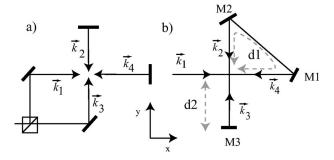
FIG. 1. 2D lattices with four beams. (a) Lattices formed by interfering two independent standing waves must be actively stabilized to be topologically phase stable against phase noise caused by vibration of mirrors. (b) Lattices formed from a folded retrore-flected beam have intrinsic topological phase stability.
