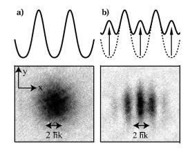
FIG. 11. (a) Single-slit diffraction pattern resulting from a loss of phase coherence among out-of-plane lattice sites. (b) Double-slit interference pattern caused by coherence between atoms within a particular double well but not among the ensemble of double wells.
