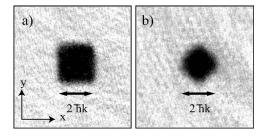
FIG. 10. Experimental images after 13 ms TOF of atoms filling the first Brillouin zone for (a) the in-plane lattice and (b) the outof-plane lattice. The shapes of the BZs reflect the momentum components in each lattice.
