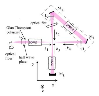
FIG. 6. (Color online) Schematic of the experimental implementation of the 2D double well lattice made from a single folded, retroreflected beam. Mirrors M1 and M2, lenses L1 and L2, and EOM $\theta$  are mounted on a fixed plate.
