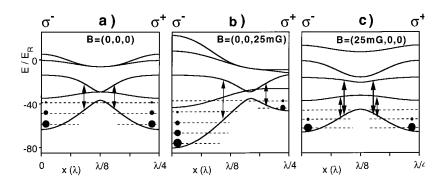
FIG. 2. Adiabatic lattice potentials for (a) no magnetic field, (b) longitudinal magnetic field, and (c) transverse magnetic field. The modulation depth of the  $m = \pm F$  diabatic potential is  $U_P = 70E_R$ , and the lattice detuning  $\Delta = -20\Gamma$ . For simplicity we show potentials for F=2; the arguments in the text apply for  $F \ge 2$ . Dashed lines and dots indicate vibrational states and their population; the arrows indicate Raman- and magnetically induced mixing.
