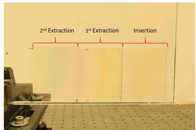
**Fig. 7.** Demonstrator showing three segments of coupling holograms named the insertion and first and second extraction holograms. Each hologram is laminated to an N-BK7 waveguide.
