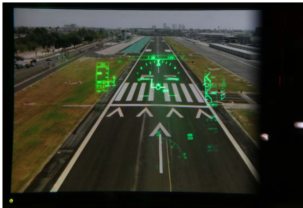
Fig. 13. Picture of the HUD system taken with a DSLR camera when focused at infinity. The background runway is displayed on a monitor located in the far field; the symbology (green) is projected at infinity through the HUD system.
