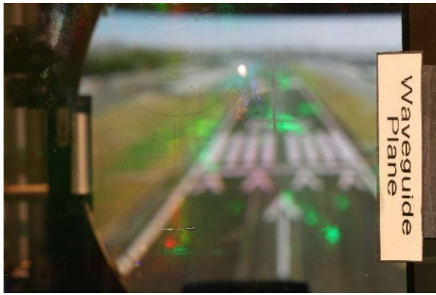
Fig. 12. Picture of the HUD system taken with a DSLR camera when focused at the location of the waveguide. The background runway is displayed on a monitor located in the far field; the symbology (green) is projected at infinity through the HUD system.
