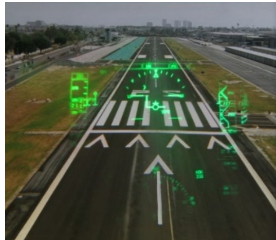
Figure 4: Picture of the HUD system taken with a SLR camera when focused at infinity. Both the background runway and the symbology projected through the HUD are in focus. This demonstrates that the viewer does not need to accommodate to see the image.
