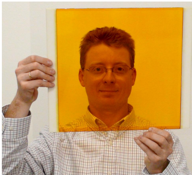
Figure 2: Large photorefractive screen for 3D display
