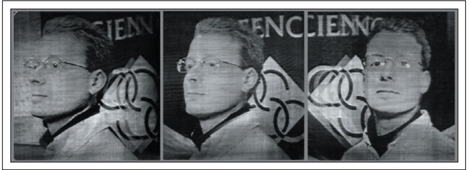
Fig. 6: A photograph of the holographic stereogram at different angles shows the parallax.
