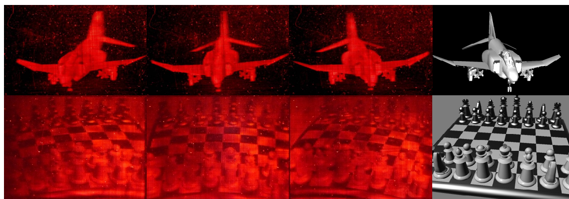
Figure 5. 2D images of the 3D holographic images produced from updatable display setup. Images are taken at different camera locations to demonstrate occlusion and parallax. The right-most images are one frame from the computer model used to generate the holograms.
