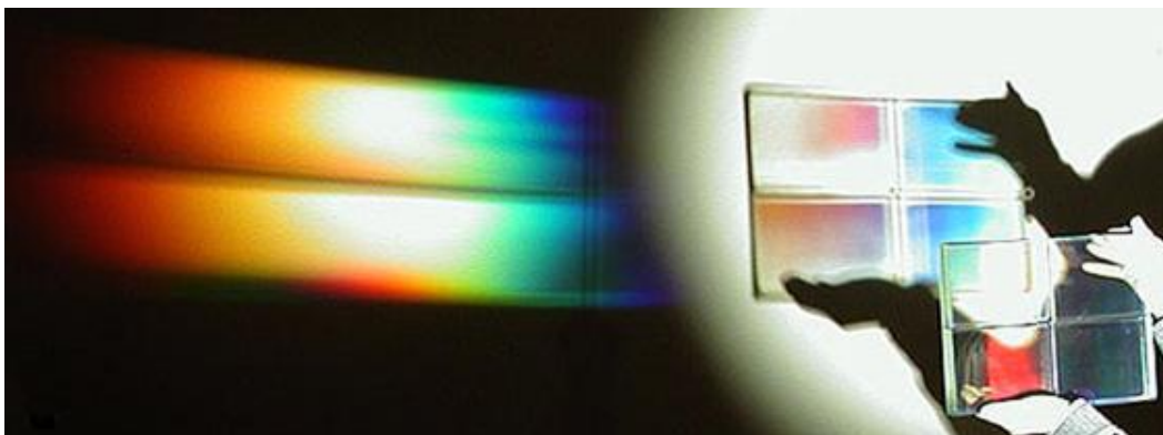
Figure 3. Picture of a 340 × 240 mm, 2 × 2 elements mosaic VPH grating produced by CSL.
