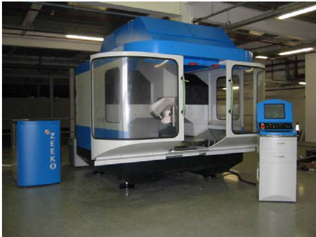
Fig. 8 Zeeko 1200mm CNC Classic/Fluid-jet polishing machine.
