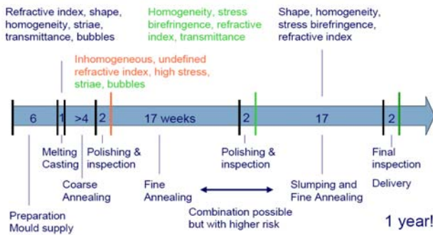
Fig. 3 Production sequence of large optical glass blanks. The lower part shows the production steps, the upper part shows when quality characteristics are defined.
