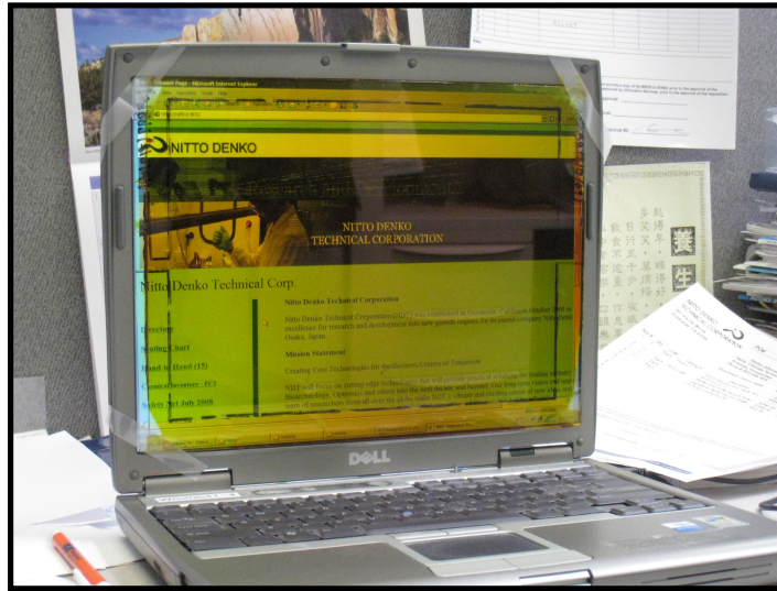
Figure 1: A 12x8 inch photorefractive device in front of a computer screen. The device is operational and has been tested to record holograms.
