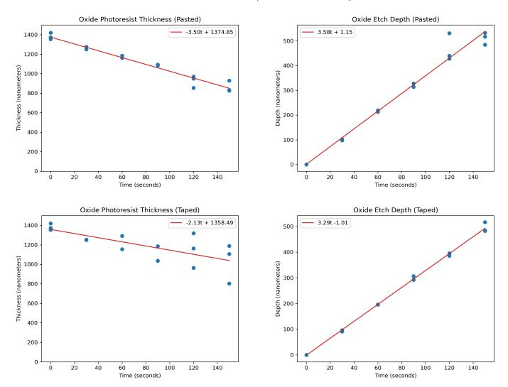
The etch rate was determined to be around 210nm/min and selectivity with S1813 was around 1.
