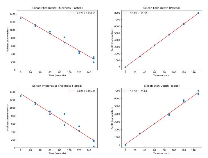
The etch rate was determined to be around 3,180nm/min and selectivity versus S1813 was around 7.6.
