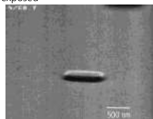
Fig.9c: 0.8 µm wide niobium dot after resist remove
