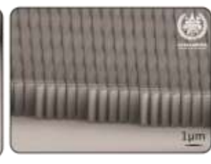
Fig.7: High AR ma-N 2410 patterns, film thickness: 1.9 µm, e-beam exposed
