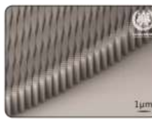
Fig.7: High AR ma-N 2410 patterns, film thickness: 1.9 µm, e-beam exposed
