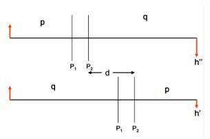
When taking this method, we need to first find one conjugate positions of object and its image. Determine the distance p and q shown in the fig. and then fix the object and image and slightly shift the optical element to find another conjugate configuration and record the distance the element move and then use these three measurement we can calculate the focal length of the optical element.
