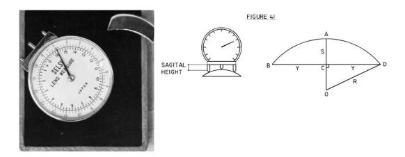
The quantity actually measured by the gauge is the sag of the surface. The dial of the gauge is calibrated under the assumption that the refractive index of the glass is 1.523. the power of the surface is given as
