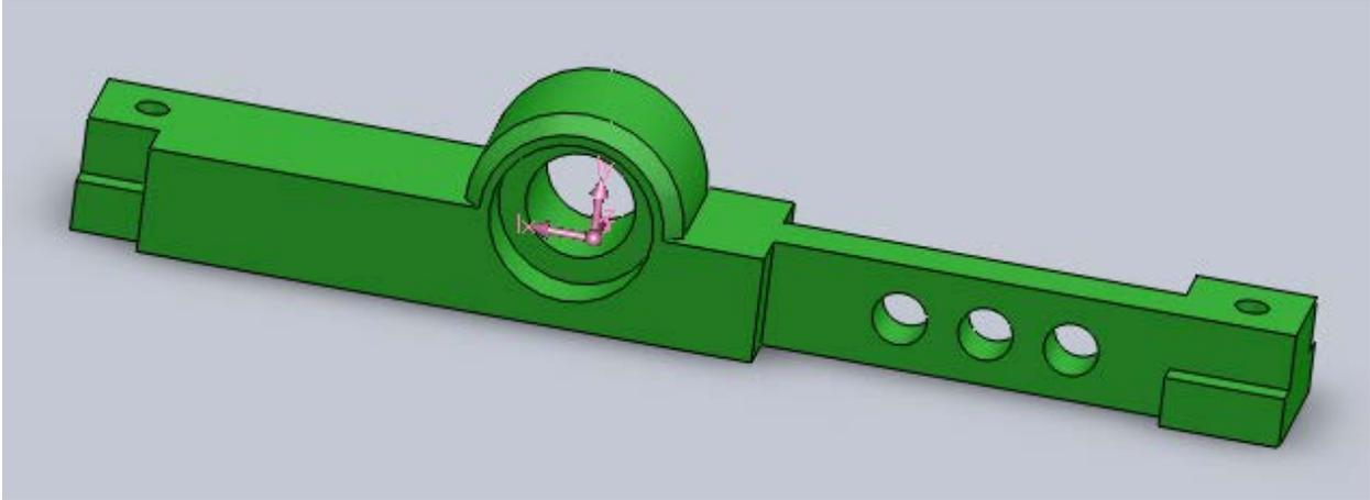
The rocker arm has a pressed ball bearing in it. The friction coefficient of a ball bearing can be approximated to be:
