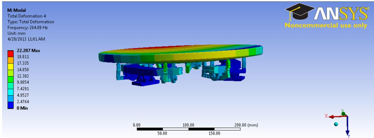
Next the piston and tilt offset was observed. The only tilt in the system is a function of the axial support since this maintains axial position. To determine the tilt the gravitational load was placed vertically and the tilt was observed by probing the axial position of the top and bottom of the mirror.
