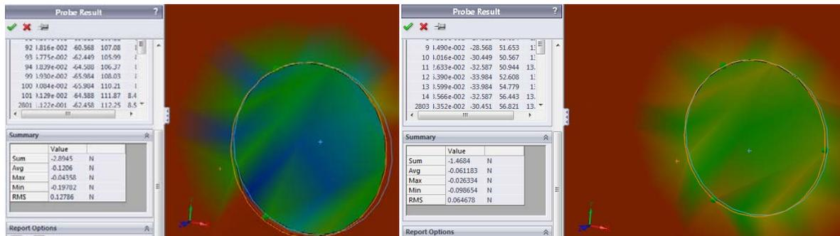
Each point in the outer ring sees a reaction force of -2.8945N. Each point in the inner ring sees a reaction force of -1.4684N. The total weight of the mirror is 26.17 N. The sum of the reaction moments adds to the weight of the mirror.
