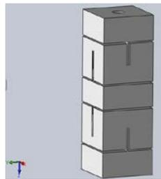
Next the tangent arms are susceptible to buckling failure. To insure this does not occur a multiple stops are positioned a distance away the edge of the mirror blank. This will insure failure does not occur under higher accelerations.
