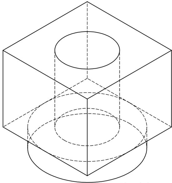
Block has a concave cylindrical radius of curvature of 12.5". The CC is aligned with center of the block. Vertex distance to the top of the block is .25in.
