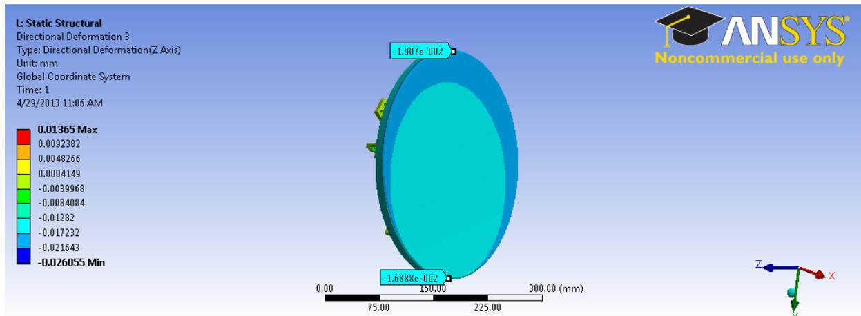
Similarly the axial displacement was determined by the maximum offset in the Z direction.
