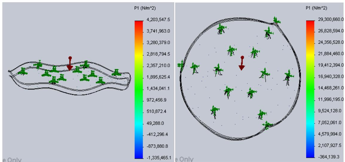
The figures about show the tangent support with 20G shock load FEA of first principal stress and axial support with a 20G shock load FEA of first principal stress. The mirror is most sensitive the lateral shock loading but will sufficiently support the mirror without failing at a factor of safety of about 1.4.
