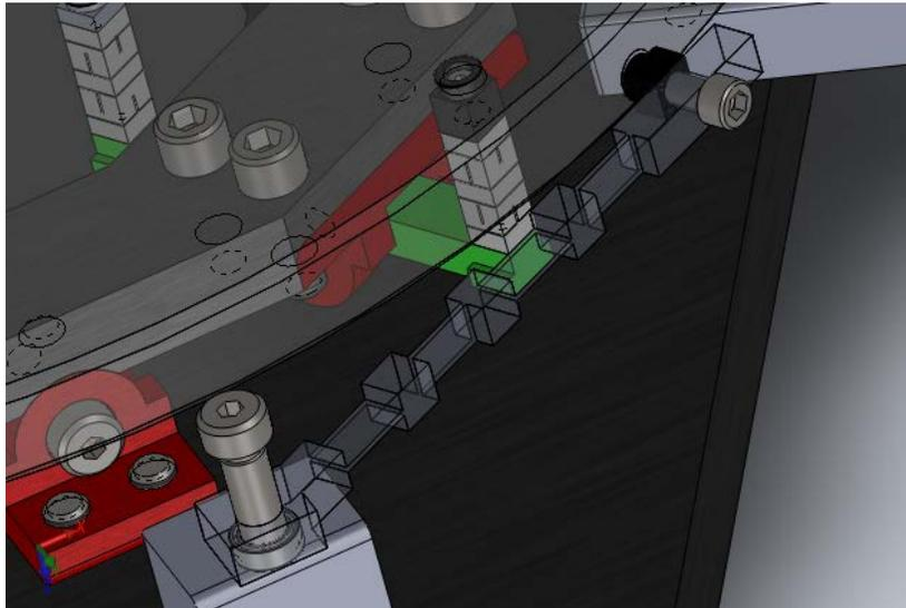
The tangent arm offers radial compliance and stiffness in lateral direction. The pivot arm is held in place by a shoulder screw that pivots about a bearing. The bearing was found necessary to this design form to minimize the frictional moment created by the pivot. The leaves in the flexure were designed such that they were thin enough to support the mirror but compliant enough to create small moments imposed on the mirror blank.
