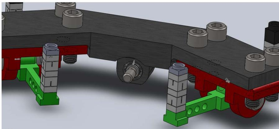
The rocker arms couple to the mirror blank via these two axis pivot flexures made of 6061 Al. The flexures are carefully designed to enable cross sectional compliance but relatively stiff in the axial direction of the flexure. The flexure axial stiffness is essential to meet system requirements.
