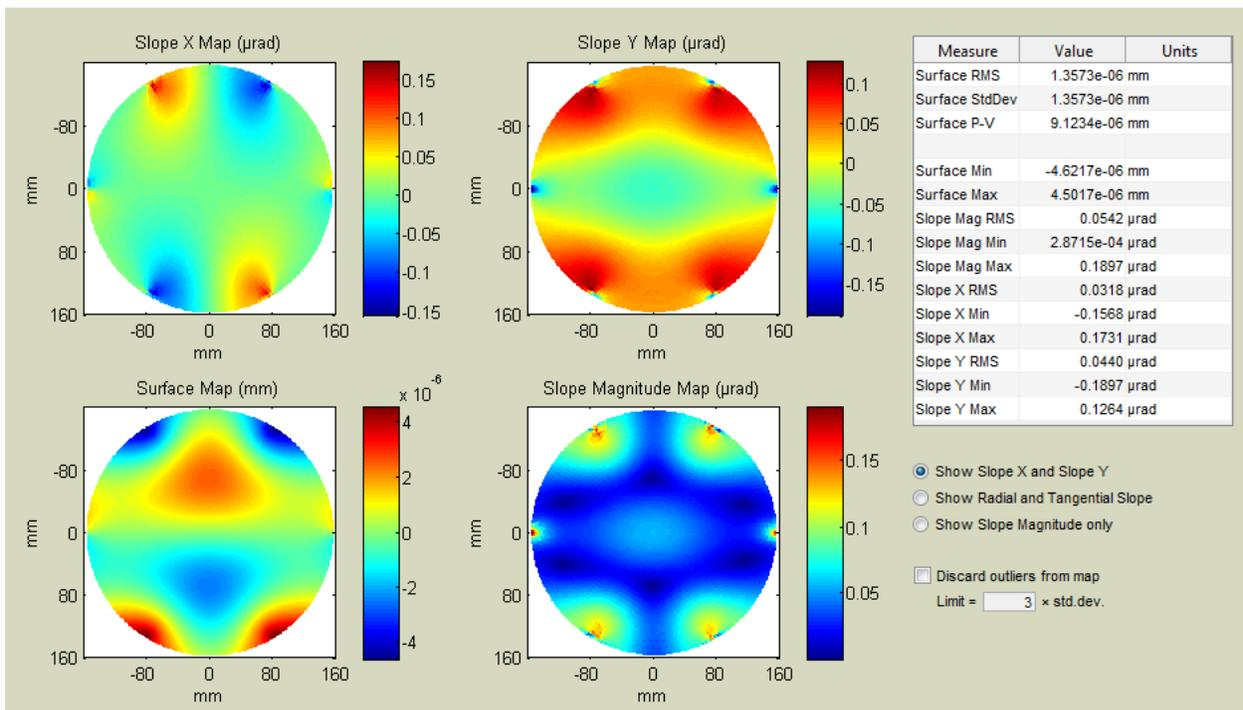
Flexure Axial Load at outer Ring
