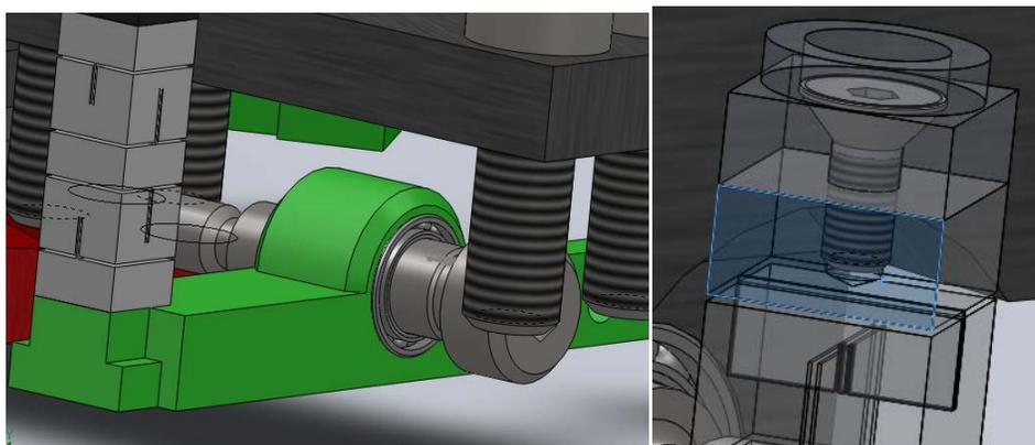
The rocker arms use precision shoulder screw to couple to the ball bearings. The ball bearings have a slight interference fit with the rocker arm. This securely holds the bearing in position after being pressed in. The pucks are pre-mounted to the flexures prior to being glued into position. This offers a relatively easy way to ensure flexures are in line with the pucks.
