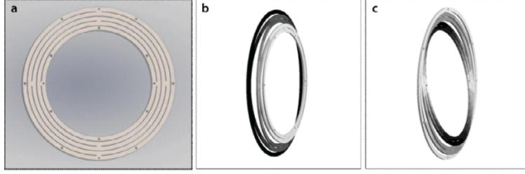
**Figure 1:** Example of a diaphragm flexure (a) shown with axial motion (b) and angular motion (c) [3].
