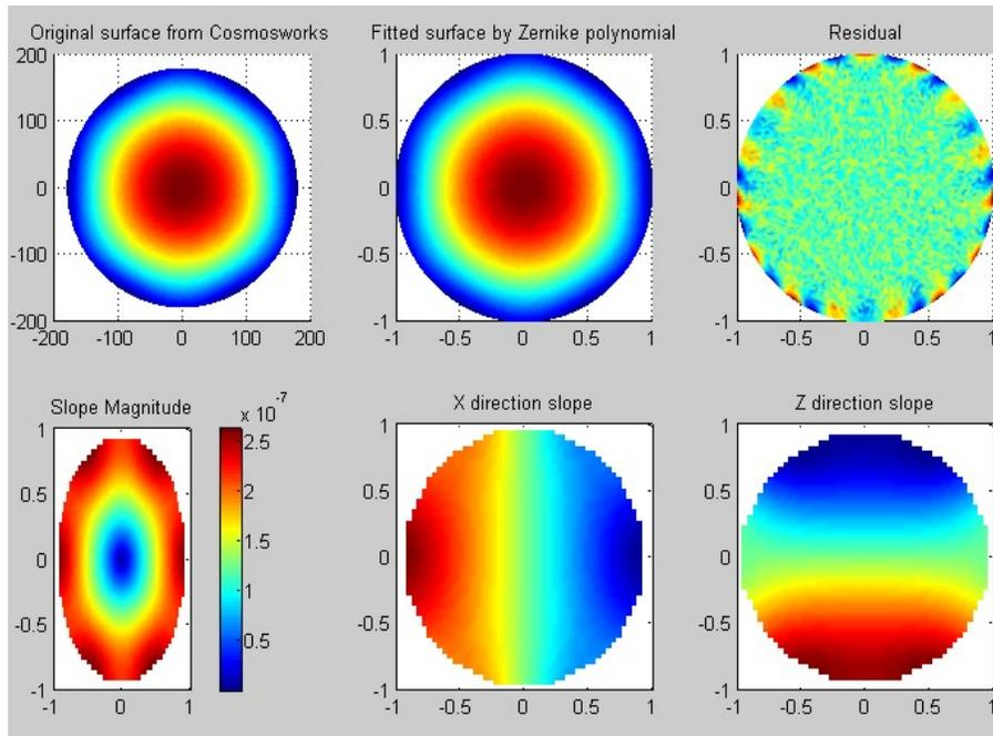
**Figure 3: Slope Error Data**
