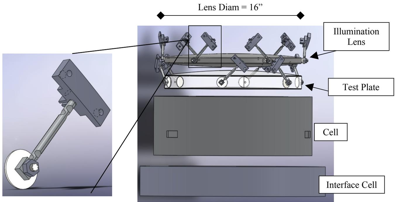
**Figure 1: Exploded View of Design Concept (top right) , close up of flexure assembly (top left), fully assembled views (below)**
