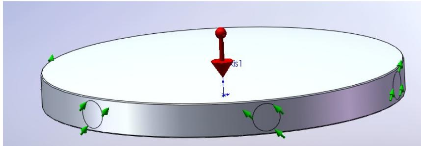
**Figure 2: Self Weight Deflection Measurement**
