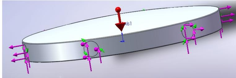
**Figure 6: Moment/Force imparted on lens by flexure**
