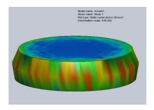
To show the radial stress distribution, a rotational part (like a slice of pizza) will be modeled with proper restraints.
