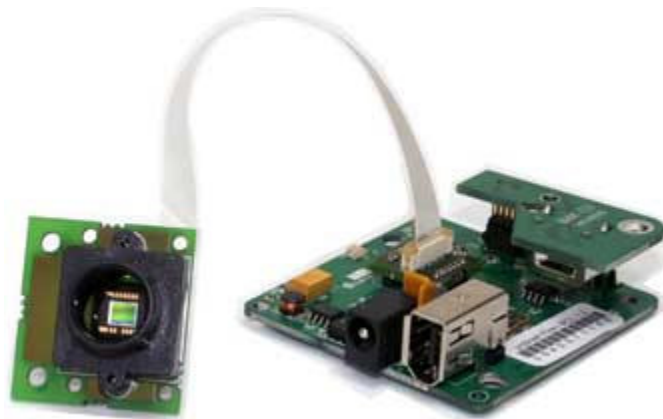
Figure 13: Digital board camera with remote CCD (Unibrain, 2009)
