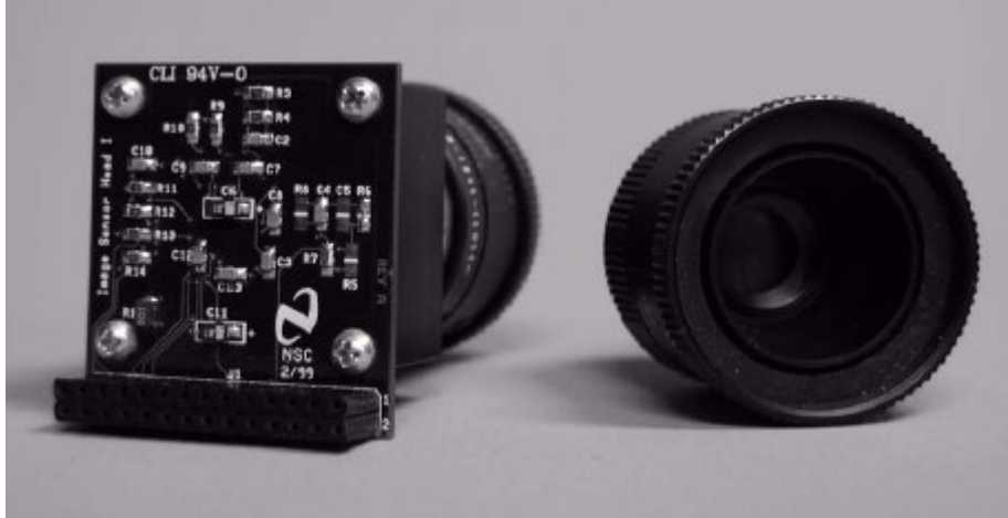
Figure 14: KAC-9618 evaluation kit headboard (Kodak Image Sensor Solutions, 2009a)
