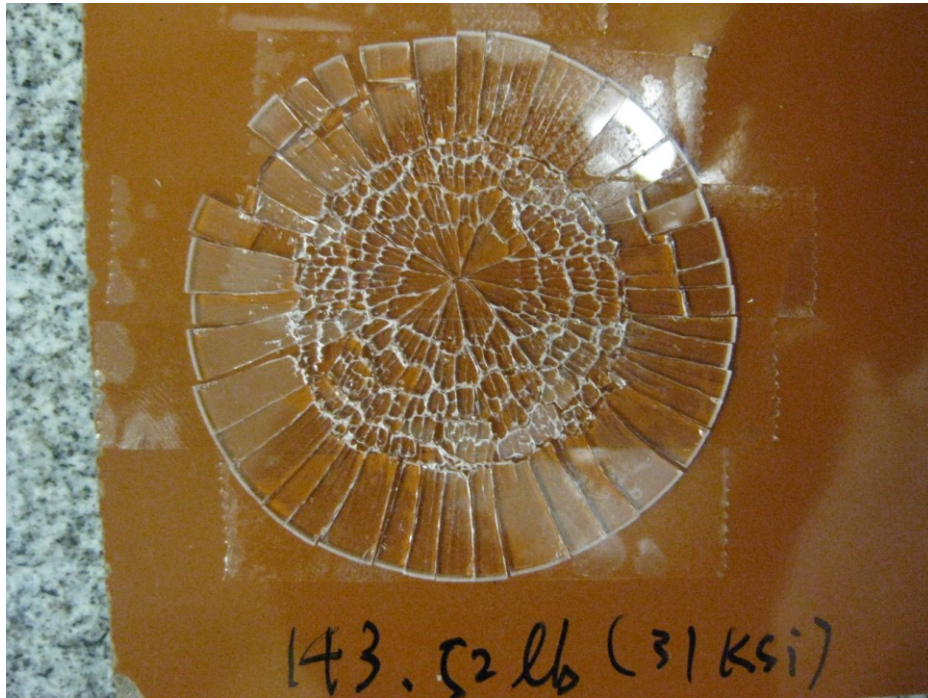
Fig 7 use double tape to hold the crack pattern of the sample
