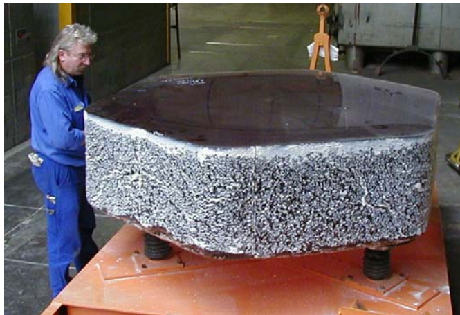
Figure 3: ZERODUR ® near net shape raw casting
