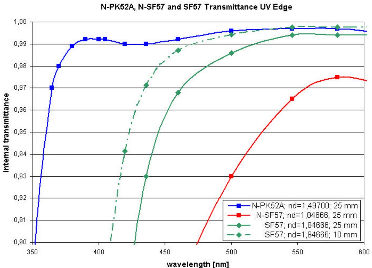
**Figure 2-3:** Catalog transmittance data of N-PK52A, N-SF57 and SF57
