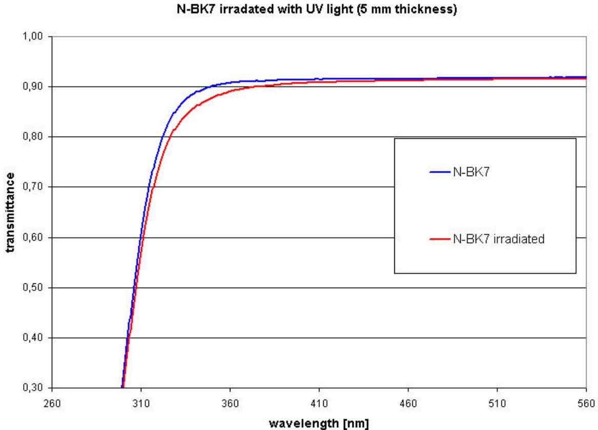
**Figure 2-5:** Solarization behaviour of N-BK7 irradiated with a HOK lamp for 15 hours.
