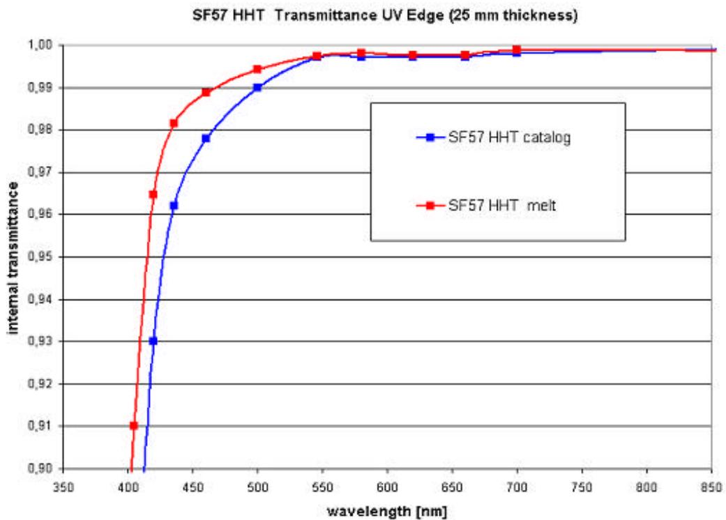
Figure 3-4: Comparison of SF57 HHT catalog specification and actual sample melt transmittance.
