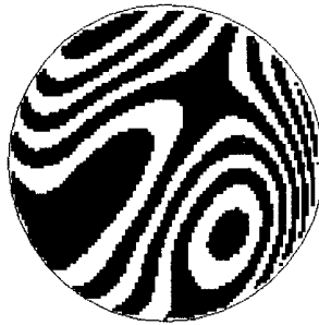
Optical surface contour interval: 0.10\lambda P-V: 0.55\lambda RMS: 0.12\lambda
