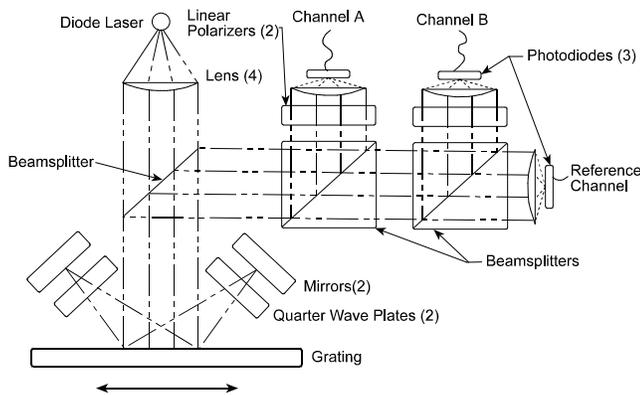
**Figure 10: Grating Interferometer Operating Principle**
