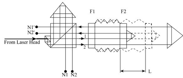
**Figure 18: Absolute Refractometer**
