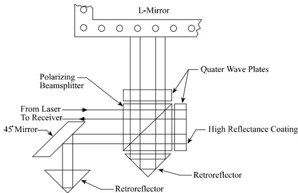
Figure 16: Four Pass Interferometer Beam Path
