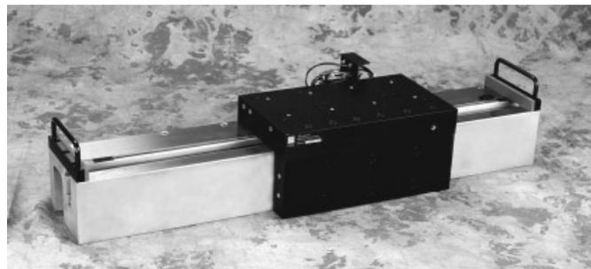
Figure 22: Air Bearing
