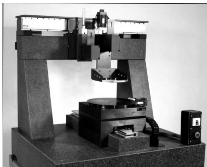
Figure 23: Air Bearing X, Y, Z System
