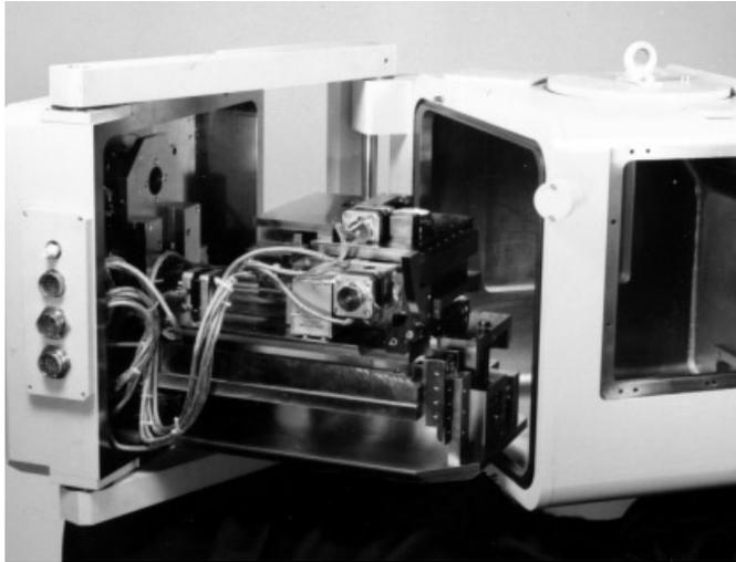
**Figure 9: Five Axis System with Grating Interferometers**
