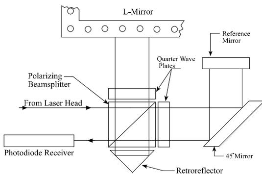
**Figure 20: Differential Interferometer**
