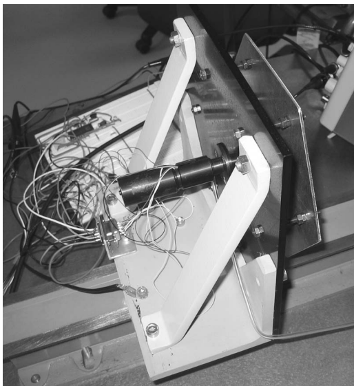
Fig. 8 Laboratory test stand with actuator and mirror simulator.
