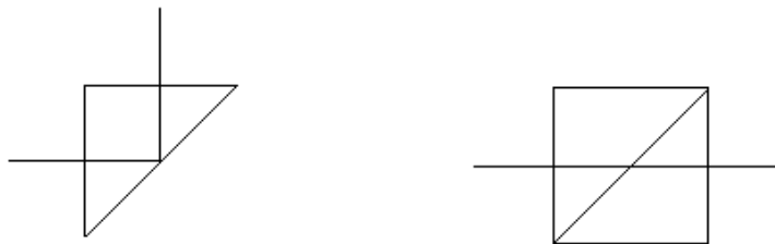
Fig. 8 Right angle prism and its tunnel diagram
