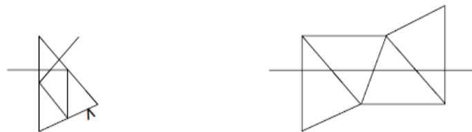
Fig. 15 Schmidt prism and its tunnel diagram
