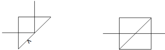
Fig. 9 Roof prism and its tunnel diagram
