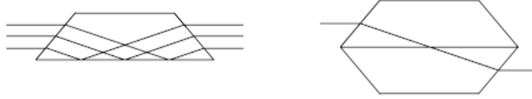
Fig. 16 Dove prism and its tunnel diagram
