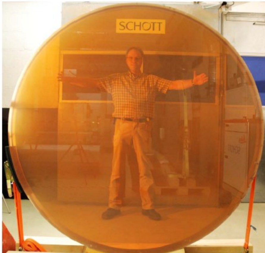
A large Zerodur blank. This picture shows the consequences of Zerodur's unusual transmittance properties.
