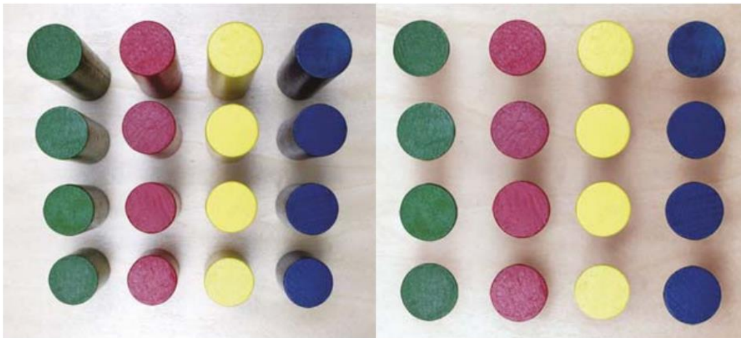
Fig 14. Photos Taken by Conventional Lens (left) and Telecentric Lens (right)
