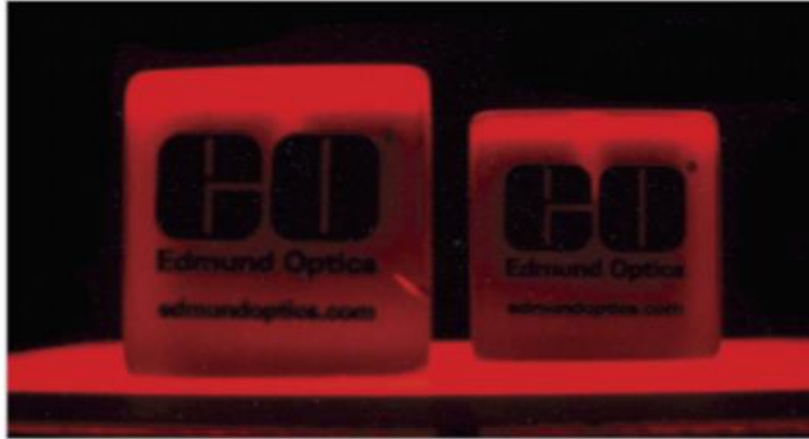
Fig 11. Photo Taken by Fixed Focal Length Lens (Angular field of view conventional lens)
