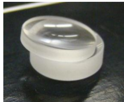
Figure 4: Ball and Socket Mount
