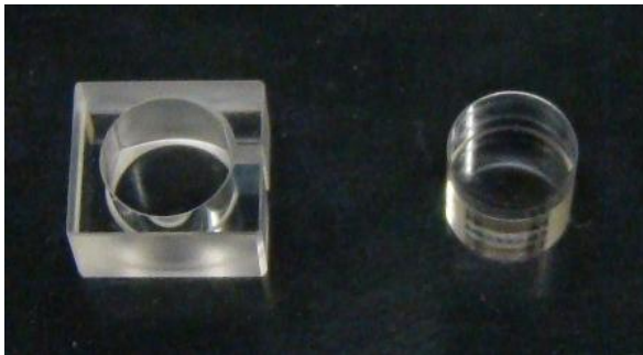
Figure 3: Split Ring and Piston Mount
