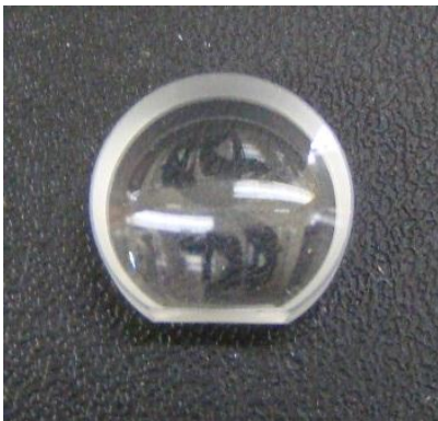
Figure 5: Edge Ground Optic for Mounting
