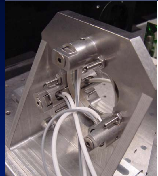
FSM Assembled and Mounted in the Test Setup
