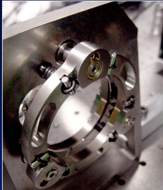
FSM Assembled and Mounted in the Test Setup
