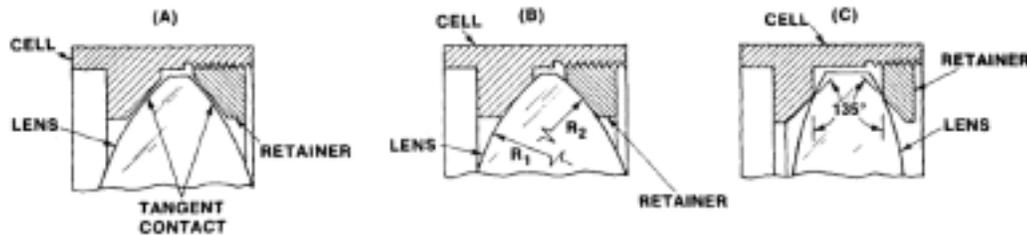
[Fig-4] Three Configurations for glass-to-metal interface
