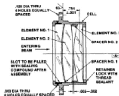
[Fig-6] a high performance telescope objective
