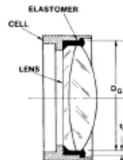
[Fig-3] Holding Lens by Elastomer
