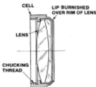
[Fig-1] Lens Burnished into a cell
