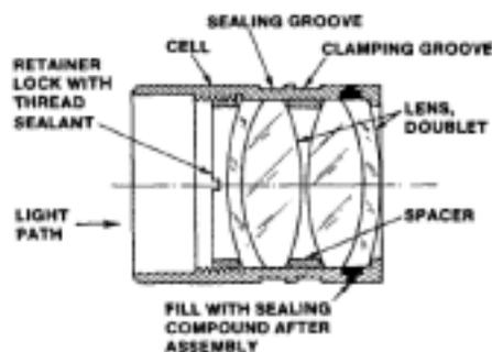
[Fig-5] Example of a fixed focus eyepiece
