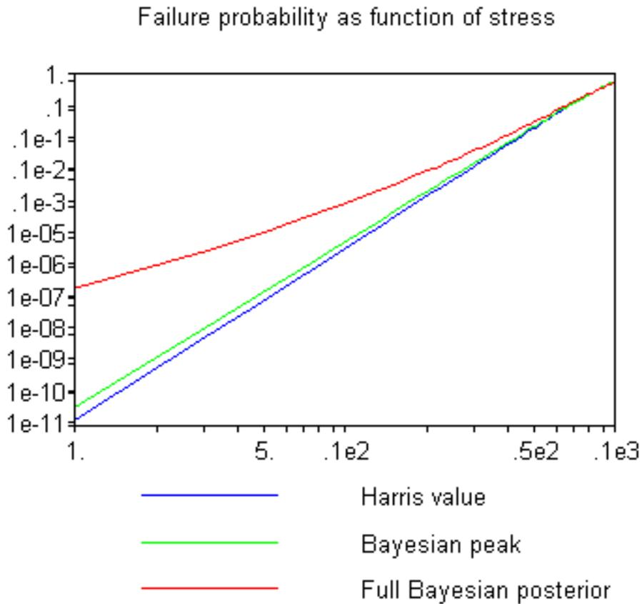
Suppose we wish to use the 13 measured failure stress values as a basis for specifying a stress level that provides a given failure probability, for disks similar to those used in the experiment. The three methods yield the following results.
