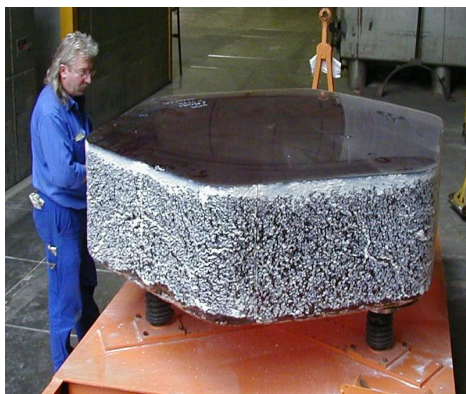
Figure 5: Raw ZERODUR cast in hexagonal shape (left) Figure 6: Achieved GTC mirror blank hexagon vertex tolerances (right)
