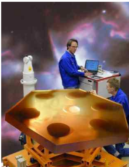
Figure 3: Measurement of GTC segments with a laser tracker system (left) Figure 4: Large CMM at SCHOTT (right)
