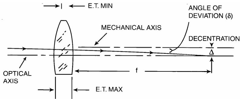
Showing the relationships between the optical and mechanical axes, and the decentration and angle of deviation in a decentered lens.
